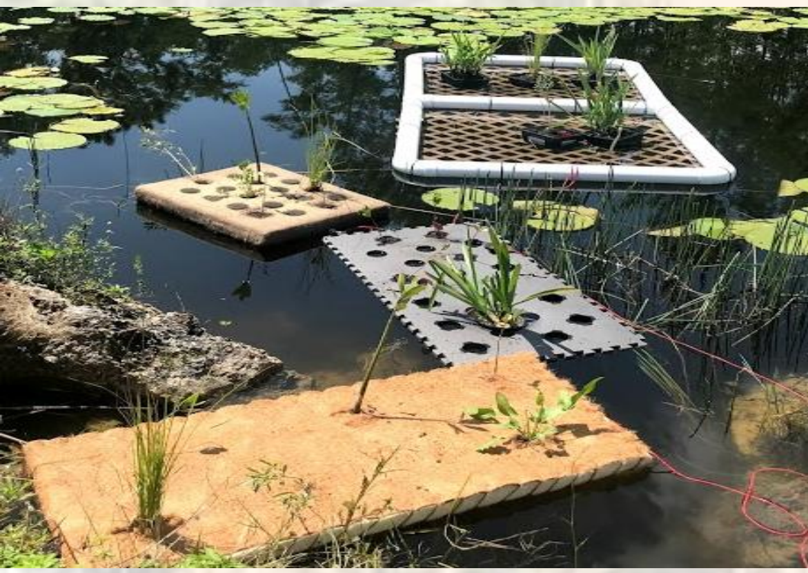
Figure 2 (above). Photo of most economical design by cost per gram of biomass supported. The 8' x 4' floating wetland cost $185.47 and is estimated to support 250 kilograms based on the volume of 4" PVC and the weight of the apparatus. The design may also support a soil component if necessary.
